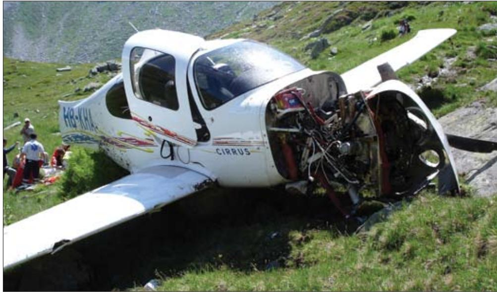
*This Swiss-registered Cirrus SR20-G2 was equipped with airbags when it crashed after entering a blind canyon in the Alps on February 7, 2006. The solo pilot suffered only minor injuries. Image provided courtesy of AmSafe.*
