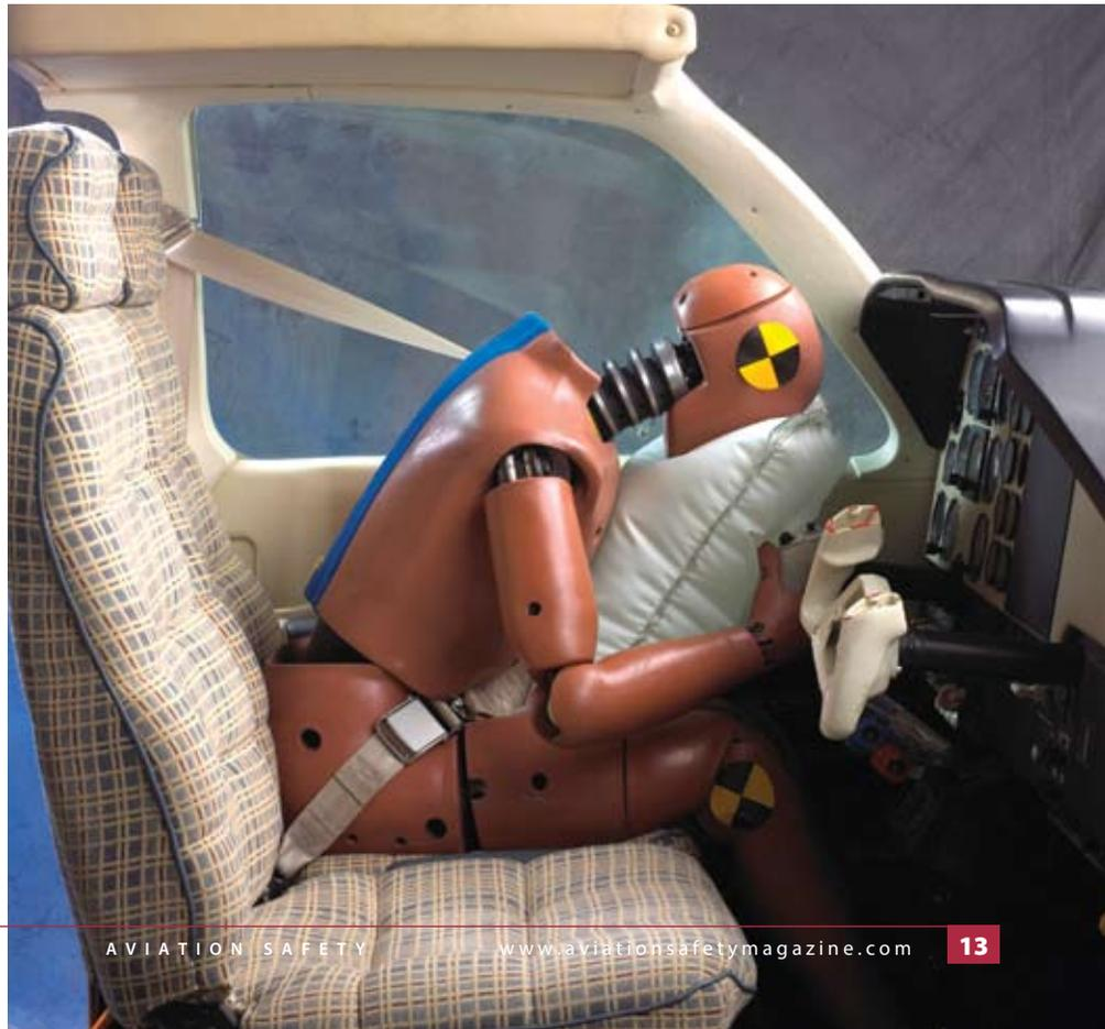
the airbag-equipped belt/harness with a hose. The EMA includes its own power source—a battery—so it is completely independent of the aircraft's systems and will function in the event of complete electrical failure. The image at the bottom of this page depicts the typical compo-
